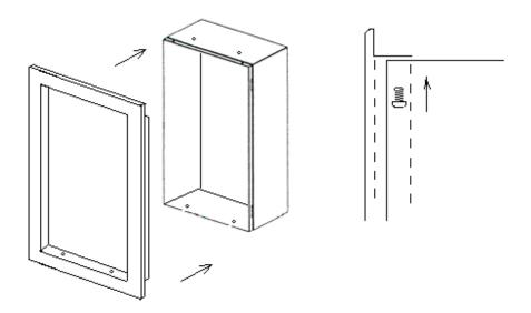
Prior to installing Door Trim, ensure that wall finishes are complete and that the door panel has been installed according to manufacturer's instructions. Verify that there is a ½" clearance from wall framing and sheet-rock or other wall surface material around the outer surface of the unit in order to permit the trim to be properly installed.
